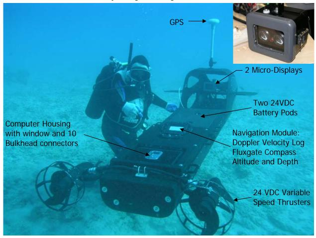
Computer Housing with Status Window and Bulkhead Connectors for Components
